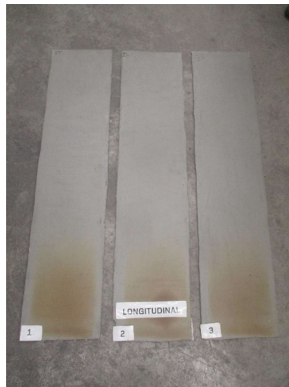
Photo n°3: Appearance of the area impacted by radiation on the three tested samples
